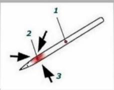
1 (Center of Gravity) different than 2 (Point of Support) and requires 3 (Grip Force Location) to Write
