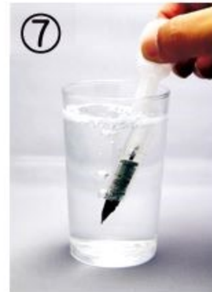
⑦ Fix an attached dropper to a nib again. Please wash it 10 times in the clean water, therefore it works better.
